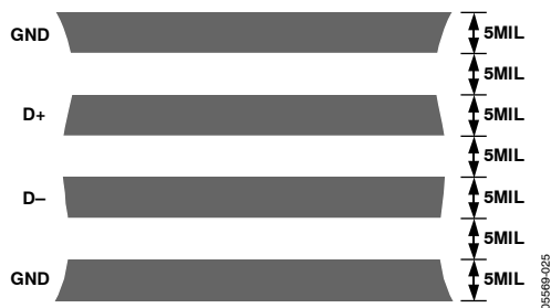
Figure 35. Typical Arrangement of Signal Tracks
